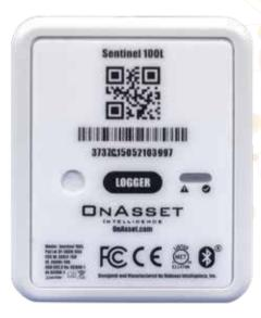
Rugged, reusable and wireless, the data logger independently logs any sensor data, and automatically offloads data to a SENTRY FlightSafe or mobile device within range - no manual process required. The Logger can store over 16,000 data points with internal memory and a 1-year battery life.
